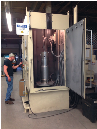
Figure 4. A simple automated blast machine for ID and OD blasting on a wide range of part sizes keeps this job shop blasting in the fast lane. Machine has multiple vertically oscillating guns and PLC controls. A crane slot with powered turntable facilitates material handling. It is shown set up for ID blasting on a jet engine burner can 13 .
