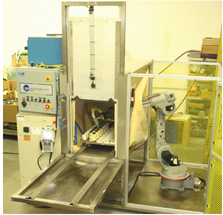
Figure 3. A work cell machine where a robot does the blasting. This wet slurry blast machine 8 is compact and clean.
